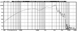
Infinite baffle response recorded at one watt at one meter.
